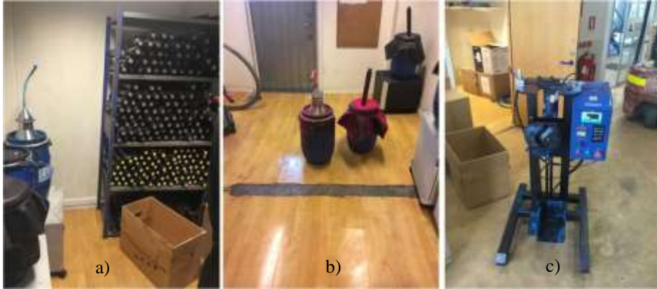
Figure 4. Equipment used for emptying and refilling toner cartridges at Company B: a) storage of sorted toner cartridges, b) barrel for recovered toner and c) refilling machine.
