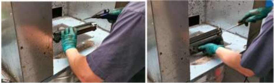
Figure 5. Cleaning and disassembling toner cartridges at Company C.
