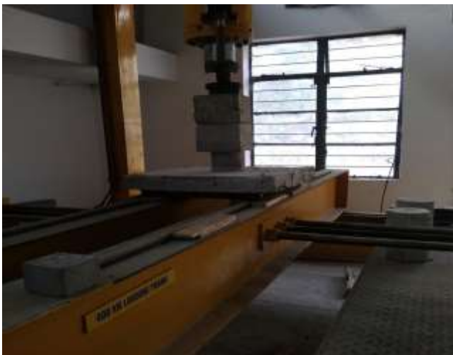
Figure 3.8.1: Slab test on the universal testing machine
