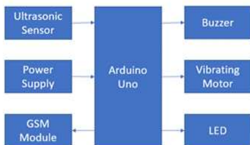
Figure 5: Block Diagram of Smart Wearable Guiding Device
