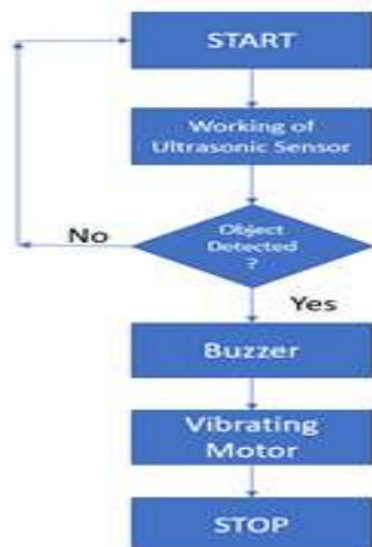
Figure 2: System Flow Chart of Smart Wearable Guiding Device
