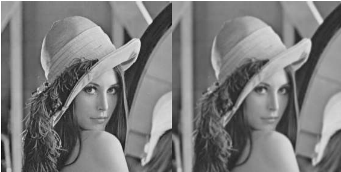
Figure 3 Left: Original image. Right: Gaussian blur with standard deviation \sigma = 2 (kernel size 13).
