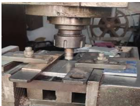
Figure 3: Plates joint process in FSW
