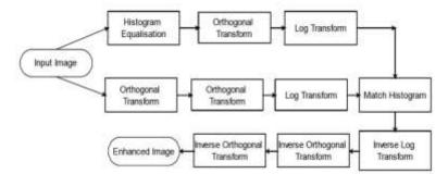
Figure 8:Block diagram of the Enhancement Processing
