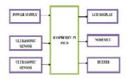
The level of wastage material in a garbage bin is detected by an ultrasonic sensor, which is HC-SR04. It is connected with the microcontroller, which is Raspberry pi Pico as shown in the Figure of the proposed system model in our scenario and ESP8266 Wi-Fi module is used to transmit the detected signal from the sensor to the Municipality office.
