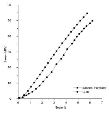
*Fig. 1: Comparison of the stress-strain behaviour of neat polyester and banana fibre composite*
