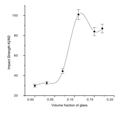
Fig. 4: Effect of resin volume fraction on the impact strength
