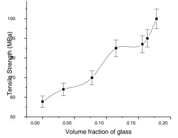
Fig. 3: Effect of glass volume fraction on the tensile strength
