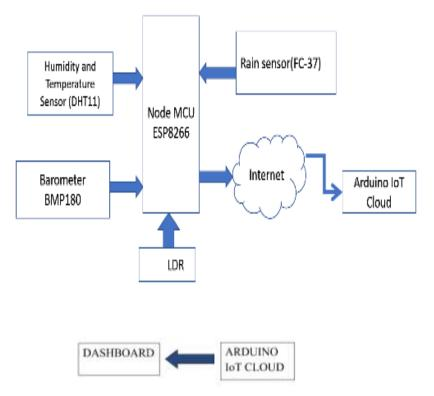
Figure 1 Block Diagram
