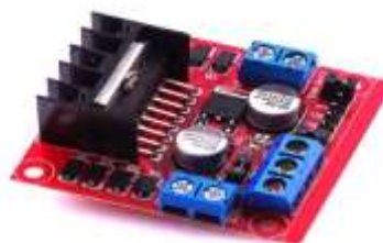
Fig 5.4 . Inverter circuit L298N
