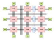
Figure.1.1. An overview of a typical FPGA architecture.
