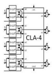
Figure 3.1 Four-bit CLA with *balanced* LUT interaction.
