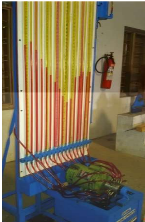
Fig.1. Experimental setup of journal bearing
