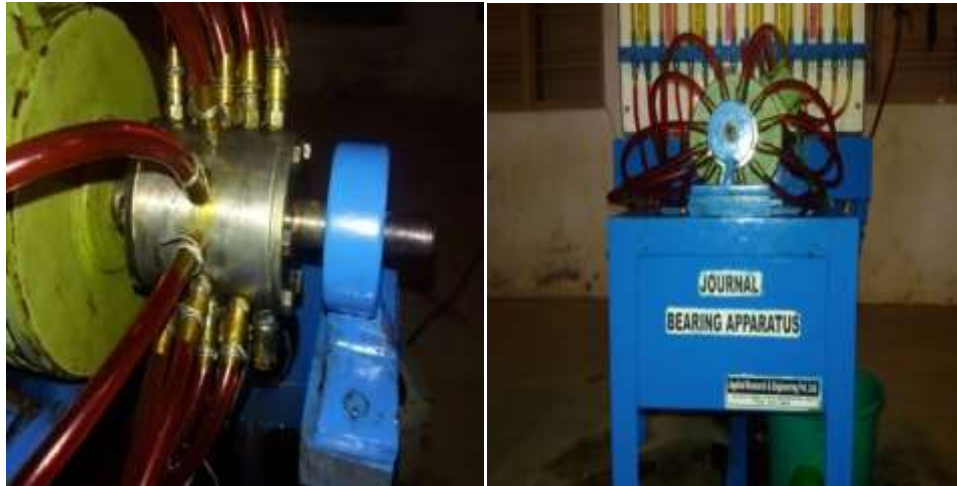
Fig.2. Manometer out lets from the Journal bearing
