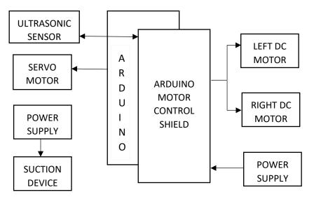
The proposed robot is a battery-operated electronic device with an ultrasonic sensor which is directed by a servo motor generates binary data. This data is then transferred to the control unit, i.e., Arduino, which is considered the robot's brain. Based on information provided by the sensor, this unit generates control signals automatically. Finally, the wheel motor drivers get these control signals.
