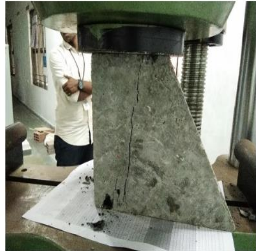
Fig. 13 Testing of END BLOCK [intrusion] in UTM
