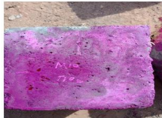
Fig. 14 Freshly Rhodamine B Dye applied specimen
