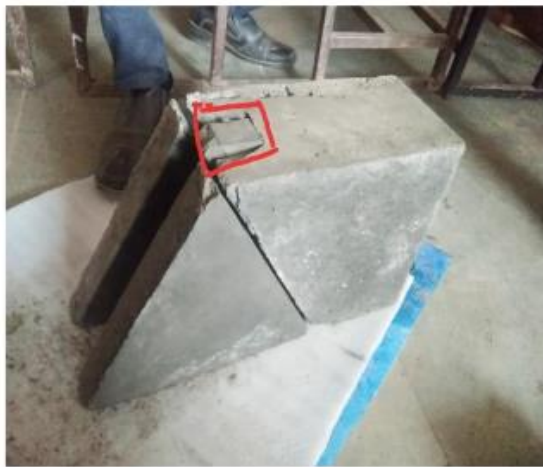
Fig.5 Image displaying small error at extrusion part with red spot.
