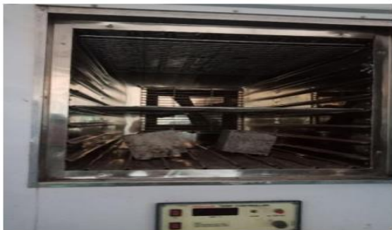
Fig.17 Specimen kept in Oven for water absorption
