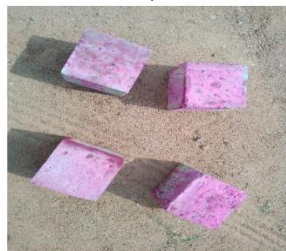
Fig. 15 Rhodamine B dye applied surface at 6 hrs.
