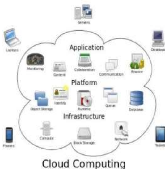
Figure1- general structure of cloud computing
