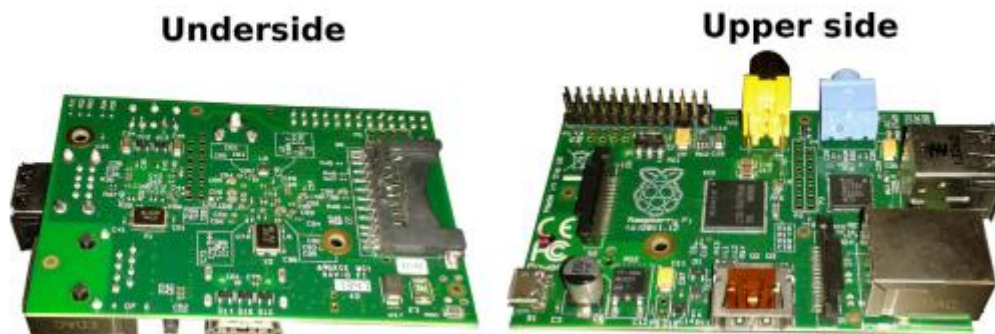
Fig. 11. Embeddable device used as a computing platform to run the PSO-PART15_ITE15 and GA-IND10_GEN25 metaheuristics to optimize the route Changing Factor parameter. This evaluation investigates whether the metaheuristics can be embedded in the UAV to reduce the rate of communication with the Control Station.
