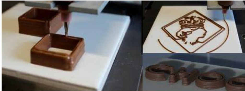
Figure 2: 3D printing of chocolate (3)
