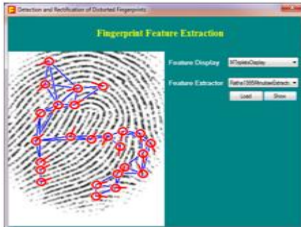
Fig.8 Minutiae-Point Marking of Fingerprint for Matching scheme using FPBA
