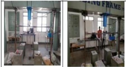
Figure 1(a). Experimental set up for loading of rolled steel bolted splice connection
