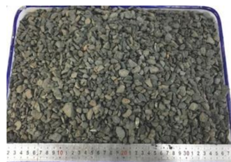
FigurE 1: Crushed shale ceramsite.
