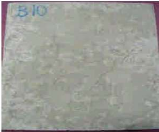
Figure 12. Reverse surface of B10 after incombustibility test.
