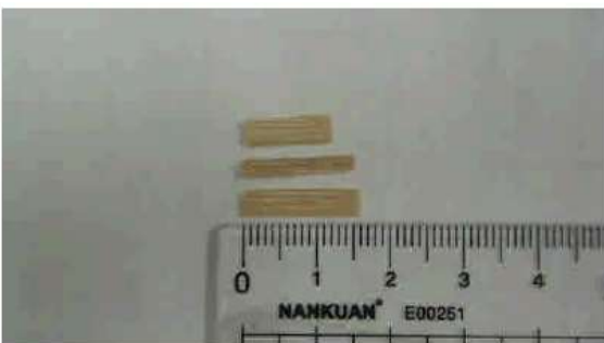
Figure 3. Bamboo fibers pass through sieve 4 and retain in sieve 8 with 15mm length.
