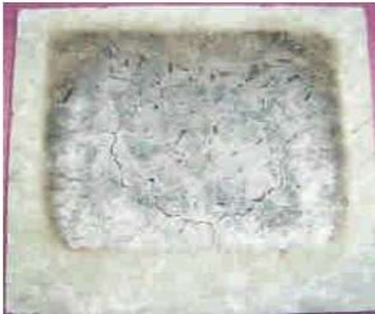
Figure 11. Heating surface of B10 after incombustibility test.
