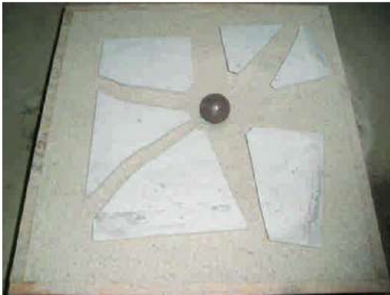
Figure 8. Fracture of counterpart material after impact test.
