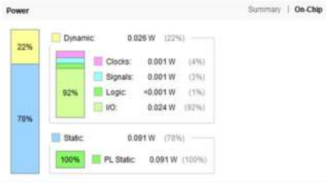
Fig.(9). Dynamic & Static power after implementation
