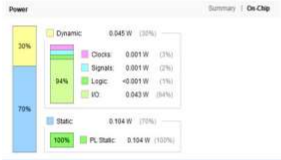
Fig.(7). Dynamic & Static power before implementation
