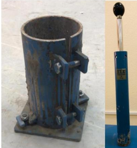
Figure 2. The mold used in preparing the specimens and the rambler that was tamping the mixture.
